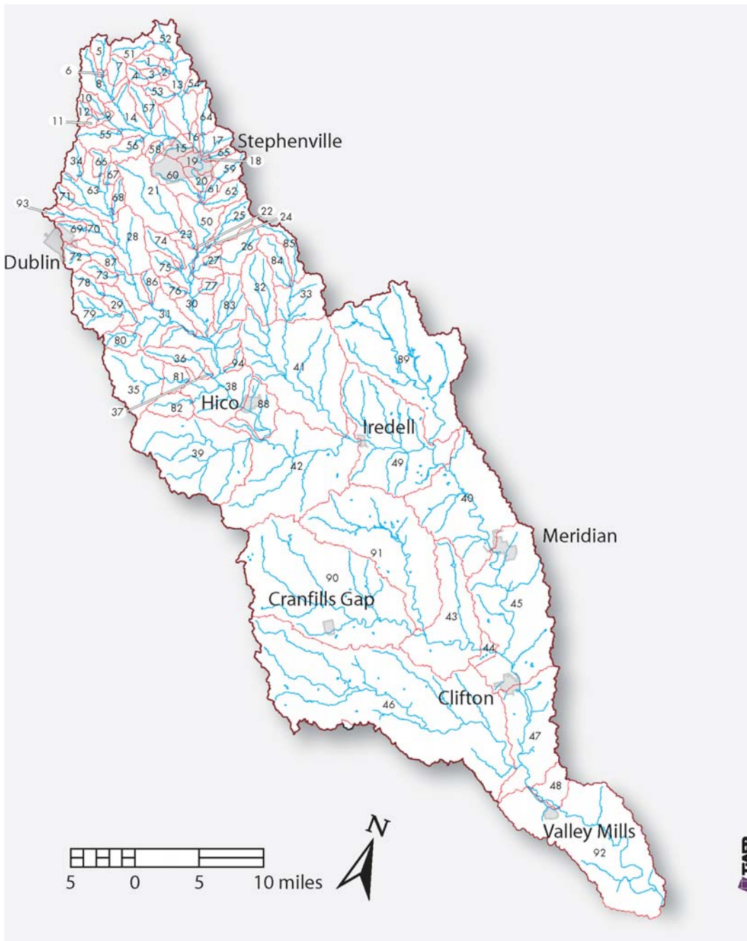
Figure 2-1 Subbasin delineation of the North Bosque River watershed used in the SWAT modeling effort. Numbers are subbasin identification numbers used by the SWAT model
