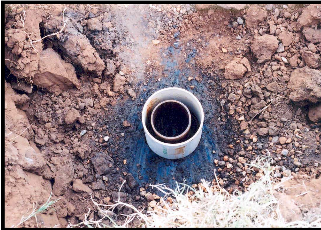
Figure 2.24 View of Double-Ring Infiltrometer in Trench 14
