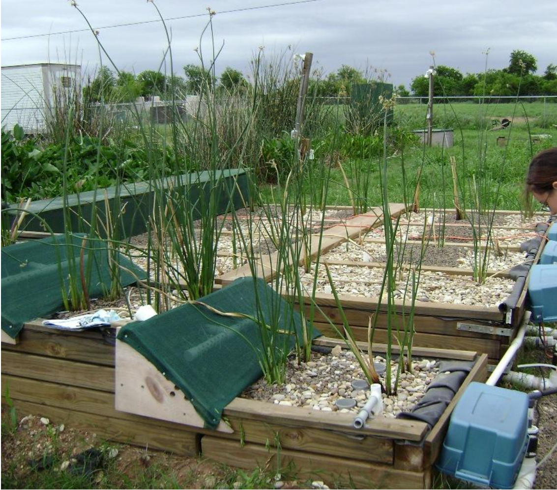
Figure 2. Photo of experimental SSF units. The units are shown in reverse order; in the foreground is Unit 5 (drip), then Unit 4 (gravel only), Unit 3, Unit 2 (no plants) and Unit 1 (control). Note the big wetland in the background left.
