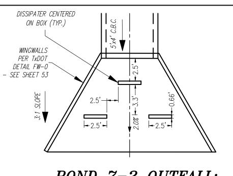
POND 7-2 OUTFALL: 5'x4' C.B.C. HEADWALL <u>DETAIL</u> N.T.S.
