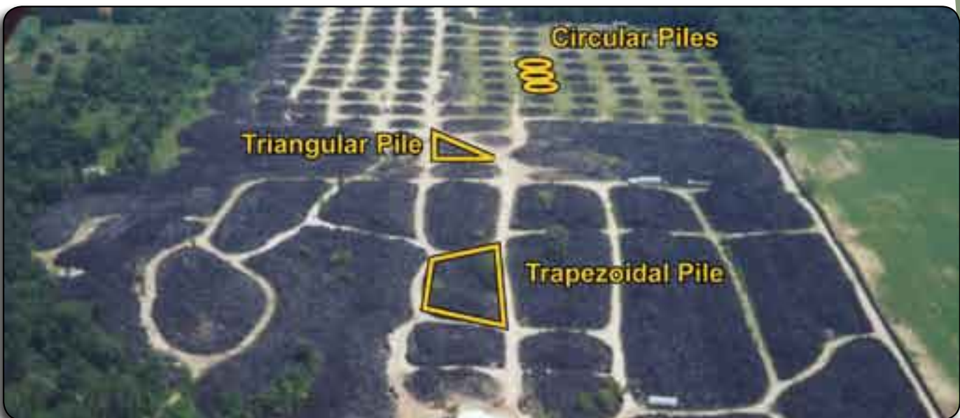
Determination of tire stockpile volume
