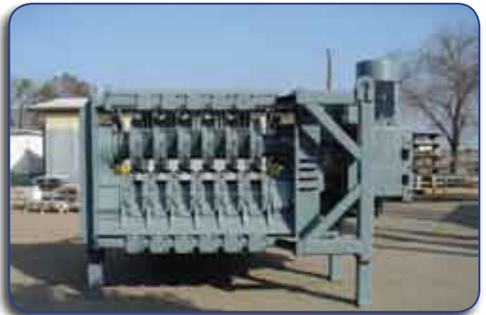
Exhibit 6-3. Tire shredder with 6-inch spaced knives Photo courtesy of Barclay Roto-Shred Inc., Stockton, CA
